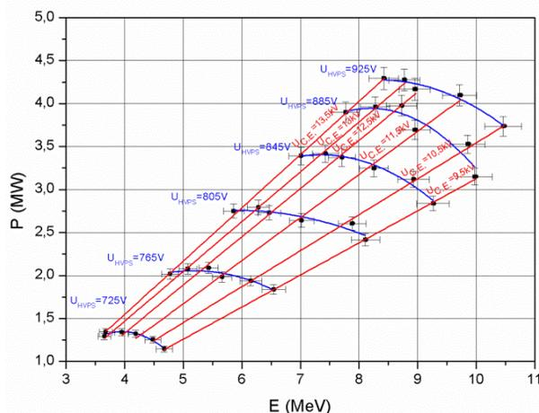
Figure 3: The relation of pulsed beam power and beam energy for the selected operation mode of the accelerator.  $U_{HVPS}$  is the charging voltage of modulator,  $U_{C.E.}$  is the electron gun control electrode voltage.
