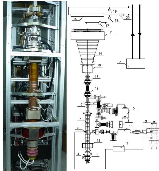
Figure 1: Photo and schematic view of the accelerator. 1 – electron gun, 2 – accelerating structure, 3 – klystron, 4, 5, 6 – vacuum pumps, 7 – low power RF unit, 8 – RF antenna, 9 – beam current monitor, 10 – scanning magnet, 11 – correcting magnet, 12 – solenoid, 13 – quadrupole lenses, 14 – scanning chamber, 15 – circulator, 16 – beam absorber 1, 17 – beam absorber 2, 18, 19 – temperature sensors, 20 – flow meter, 21 – chiller.
