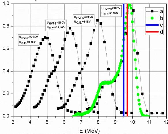
Figure 5: The beam spectra measured by the absorber 16 (Fig. 1) (a), by radiochromic film (b), beam energy from dose-depth distribution measurement (c) and from average power and pulsed current measurements (d).
