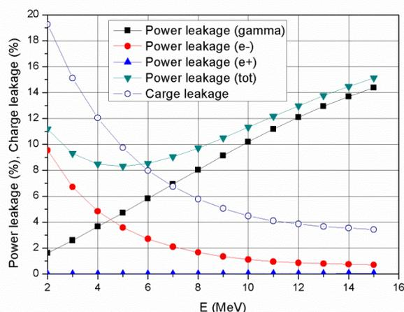
Figure 2: The dependence of the beam power and charge leakage on the electron energy due to the bremsstrahlung, secondary electrons and positrons.
