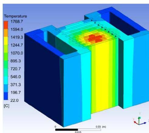
Figure 4: The temperature distribution in target with 5 cm in height ( $D_H = 15.65 \times 10^{-3}$  m,  $v = 2.5$  m/s).
