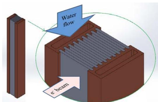
Figure 3 : Schematic view of target and cooling ducts.
