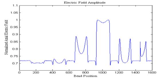
Figure 5: The measured axial electric field profile before frequency tuning.
