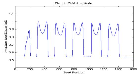
Figure 6: The measured axial electric field profile after frequency tuning.
