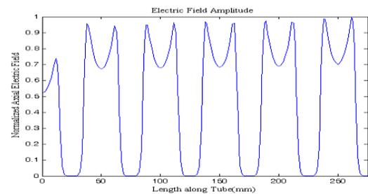
Figure 7: The simulated axial electric field profile.
