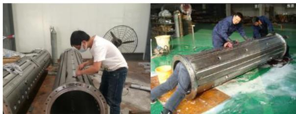
Figure 4: Surface acceptance and degreasing.
