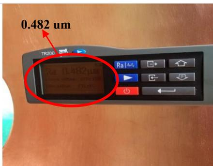
Figure 5: Plating thickness measurements and surface roughness measuring.
