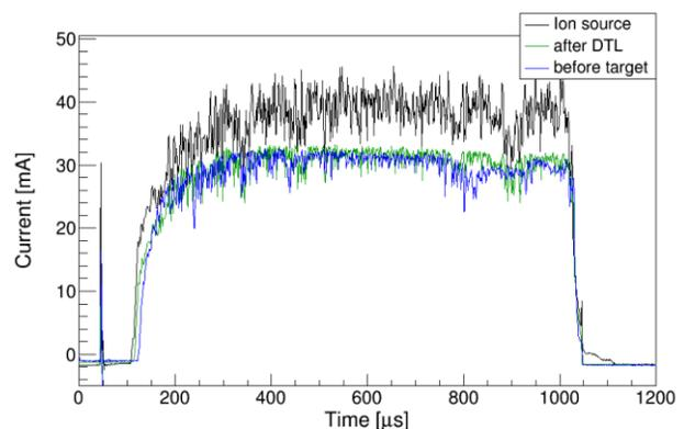
Figure 1: Waveforms taken with CTs installed at the ion source (black), after DTL (green) and before the target (blue), respectively.
