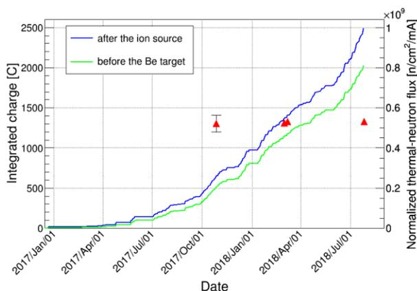
Figure 2: History of the amount of integrated charges after the ion source (blue) and the beam transport line before the target (green), respectively. Triangle plots indicate the thermal-neutron flux normalized the current.
