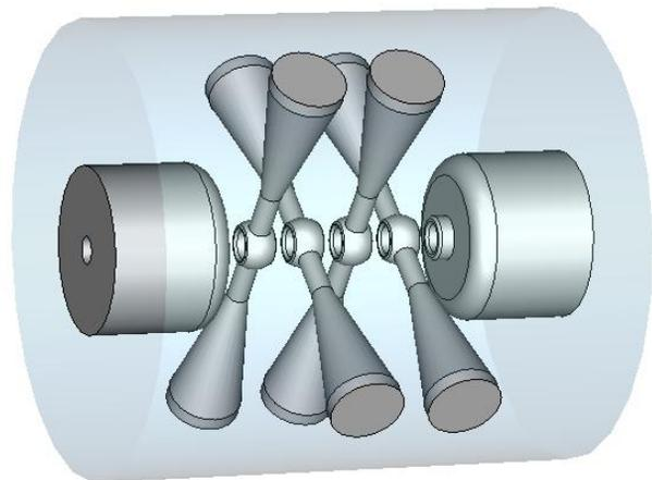
Figure 6: 3-D geometry of the 5-cell CH-DTL cavity model.
