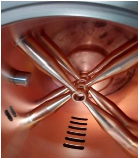
Figure 9: The inside view of the manufactured cavity.
