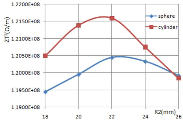
Figure 5: Shunt impedance for two different drift tube shapes as a function of the stem-base radius.
