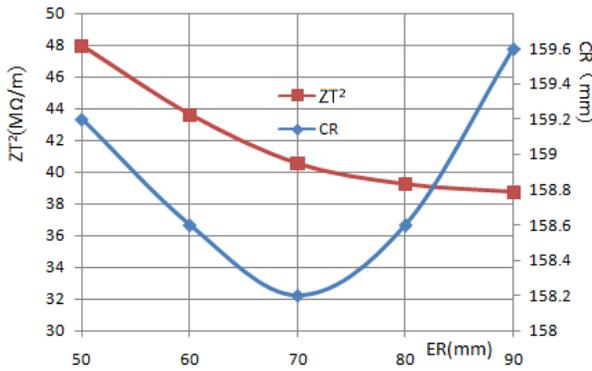
Figure 7: Shunt impedance and cavity radius at a fixed frequency as a function of ER for a 5-cell cavity without end cups.
