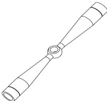
Figure 4: Spherical drift tube.
