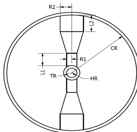
Figure 1: Geometry of a CH single cell.
