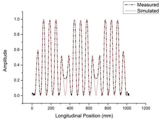
Figure 3:  $E_z$  distribution along Z direction.
