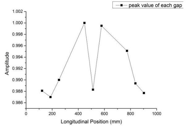
Figure 5: The peak value of 9 drift tube gaps.
