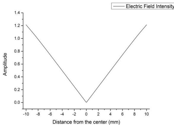
Figure 4: Electric field distribution along the angle bisector of quadrant at the RFQ section.
