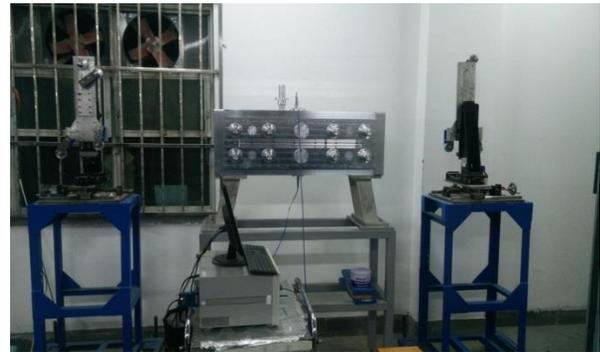
Figure 2: Bead-pull measurement system.
