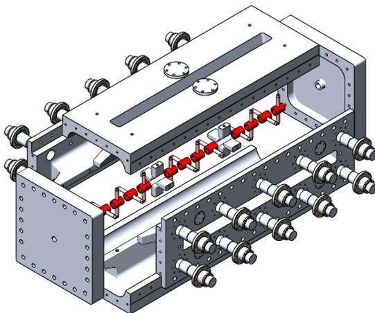
Figure 1: The overall mechanical model of Hybrid RFQ.
