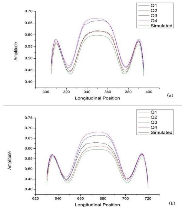
Figure 6: Quadrupole field distribution. (a) shows the first set of quadrupole. (b) shows the second set of quadrupole.
