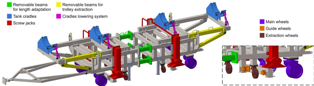
Figure 4: Design of the Tank Handling Trolley (THT).
