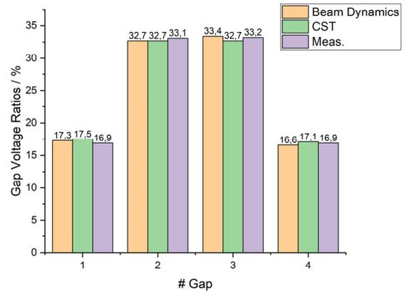
Figure 4: Comparison of the gap voltage ratios for CH 2.
