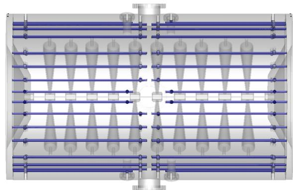
Figure 5: Cooling system of CH 8 tank (side view).
