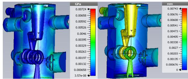
Figure 11: Von Mises Stress and displacement due to 1 bar pressure on the rebuncher external wall (internal vacuum) and self-weight assuming the auxiliary system will be supported independently neglecting the residual moment on the rebuncher-supported around the surrounding of the chamber bottom wall.
