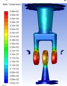
Figure 6: Temperature map on inner surface of the rebuncher due to 5 kW dissipated power (left) utilizing central cooling configuration basic model (right). All surfaces with a temperature increment less than 2 K are filtered out.
