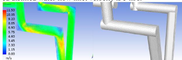
Figure 12: The fluent velocity path (left) for the derived 4 mm cell mesh-length (right)
