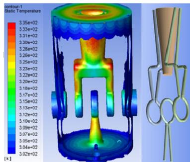
Figure 8: The Rebuncher temperature map for the derived cooling configuration with 4 cooling lines and a coaxial cooling cone at the top fork top cone and a cooling line for the central drift tube due to 20 kW dissipated power.
