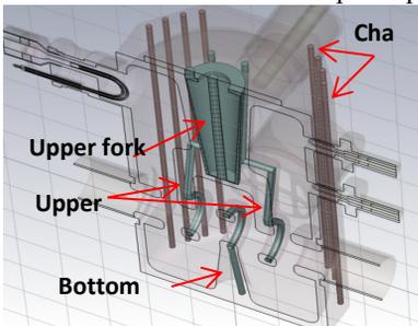
Figure 9: The rebuncher finalized engineering design with the integrated derived cooling configuration.
