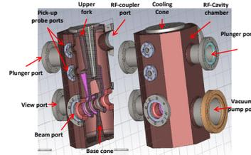
Figure 1: The rebuncher design.
