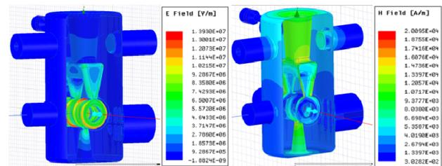
Figure 3: The induced surface electric field (left) and magnetic field (right) for 20 kW input power received with the driven modal HFSS solver.
