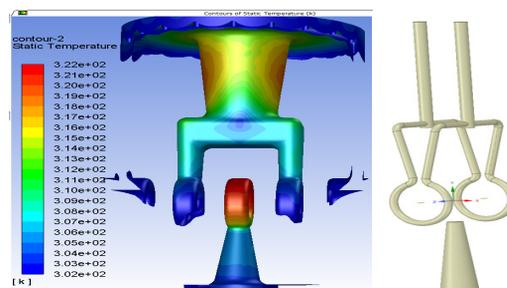
Figure 7: Rebuncher temperature map with two cooling pipes in the central stem and cooling lines in the top drift tubes due to 5kW dissipated power.
