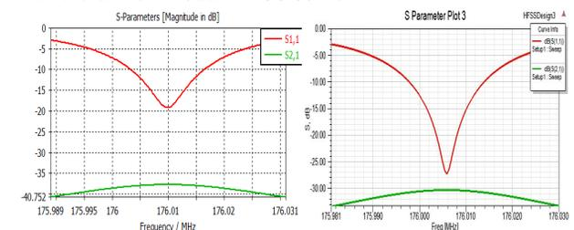
Figure 4: S-parameters of the rebuncher results from driven modal solvers of CST (left plot) and HFSS (right plot) - S11 (red curve) and S21 (green curve). The frequency range is the FWHM value (S21 -3dB level).
