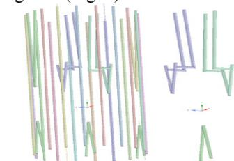
Figure 5: Basic cooling geometry: main chamber + central bodies (left) central bodies only (right).
