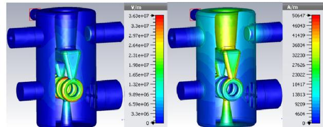
Figure 2: The induced eigenmode surface electric field (left) and magnetic field (right) at 176 MHz normalized for a 1 Joule rebuncher stored energy received from CST MW studio.
