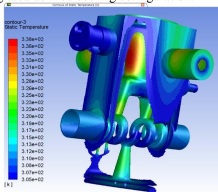
Figure 10: The rebuncher temperature ANSYS Fluent map for 20 kW dissipated power assuming reasonable distilled cooling water velocity of 5 m/s demonstrate modest temperature rise of 38 K.
