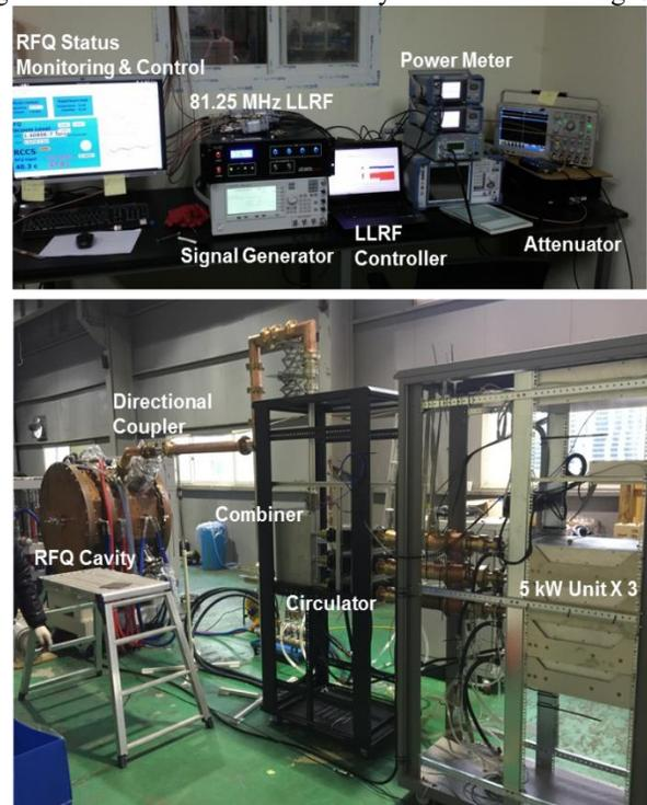
Figure 2: Test setup with 81.25 MHz LLRF, 15 kW SSPA and RFQ cavity.
