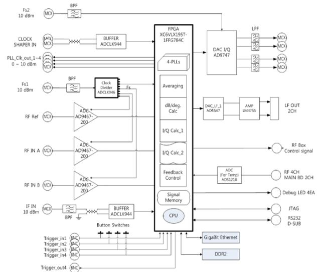
Figure 1: Block diagram of 81.25 MHz LLRF module.
