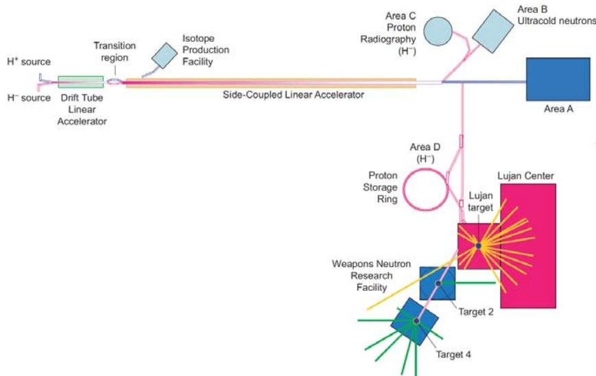
Figure 2: Graphical representation of the LANSCE accelerator.
