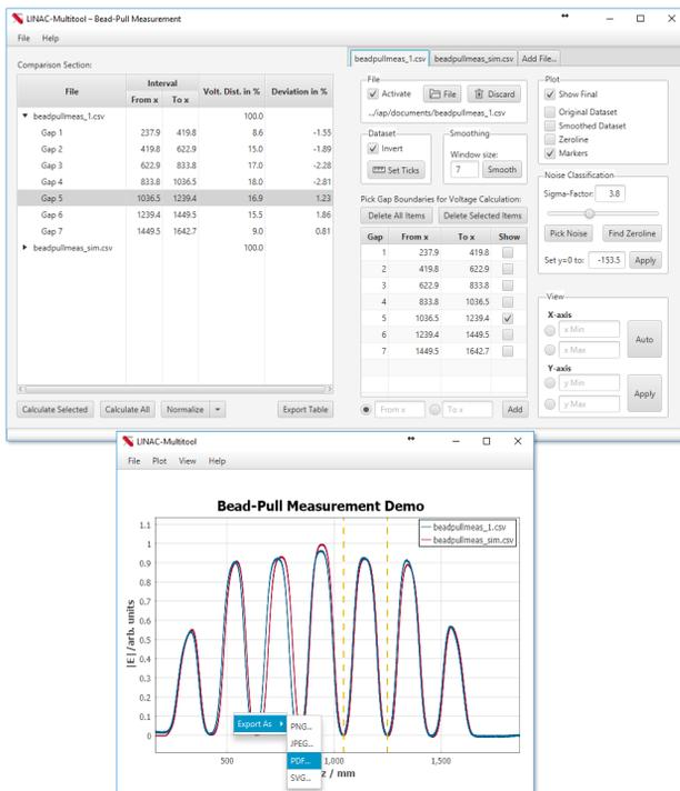
Figure 4: Screenshot of the bead-pull measurement GUI.
