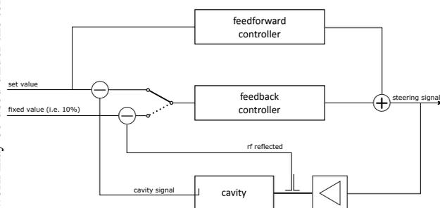
Figure 3: Basic block diagram of the foreseen controller with the feedforward controller and the feedback controller. When the cavity is out of resonance i.e. during startup phases, the reflected rf power is used as the reference value.
