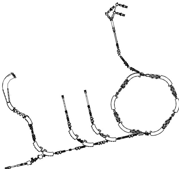
Figure 1: The accelerator of the Heidelberg Ion-Beam Therapy Center (HIT) with three ion sources, the LINAC (7 MeV/u) consisting of a 4-rod-RFQ and a IH-DTL, the synchrotron (48-430 MeV/u), the beam lines to the treatment rooms and the experimental area and the heavy ion gantry [2].
