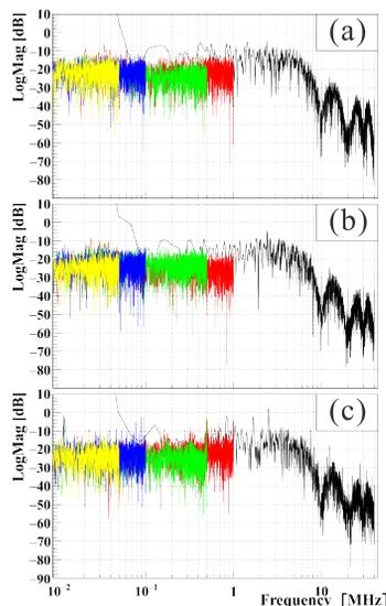
Figure 4: FFT results of (a) ADC1 channel, (b) ADC2, and (c) ADC5 with the condition of DFB using ADC1.
