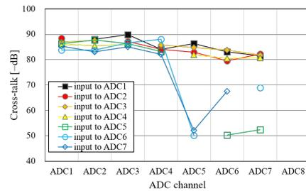
Figure 2: Cross-talk level in the new board. The  $-50$  dB cross-talk level was obtained in the case of the 324 MHz RF signal inputted to ADC5 to 7. However, the ADC1 to 4 channels for the use of DFB were estimated to have the insignificant effect.
