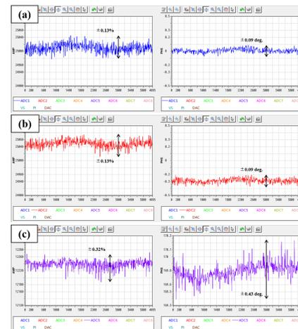
Figure 3: Stabilities of amplitude and phase for (a) ADC1 channel, (b) ADC2, and (c) ADC5 with the condition of DFB using ADC1.
