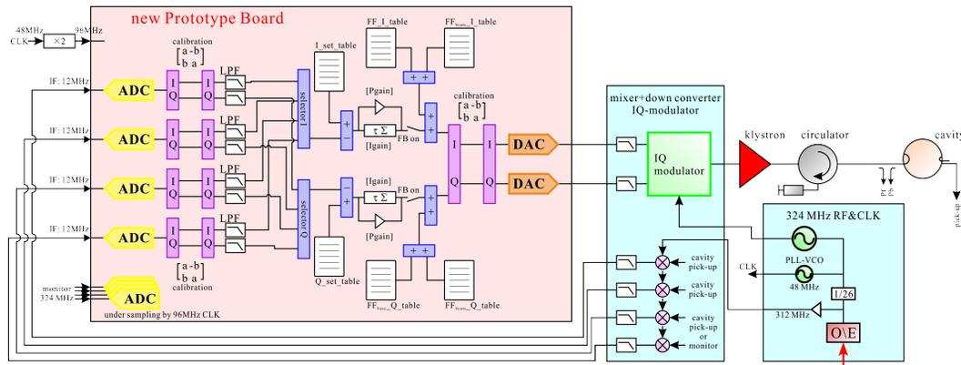
Figure 1: Block diagram of the new prototype board. The red hatching region is the new prototype board, and the modules of the sky blue region, RF&CLK board and mixer&IQ-modulator, of the present cPCI are used in the first step.
