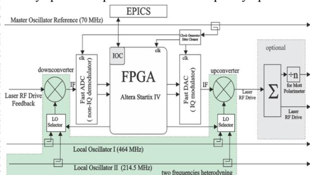
Figure 2: One channel of the Laser LLRF.
