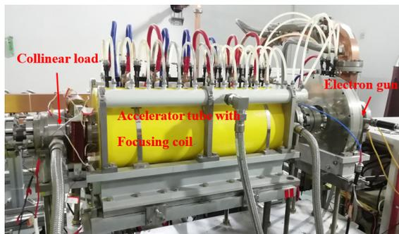
Figure 3: The HUST-FEL-THz injector equipment.
