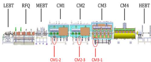
Figure 1: The layout of ADS 25MeV linac.
