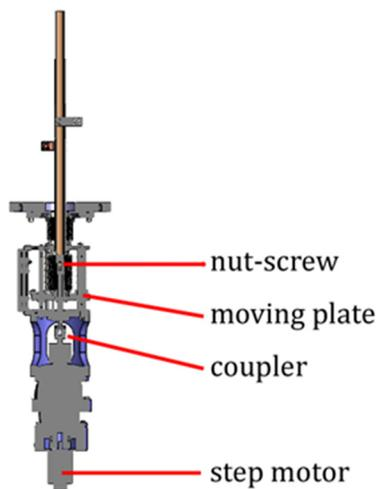
Figure 2: The sectional view of the tuner linear part.
