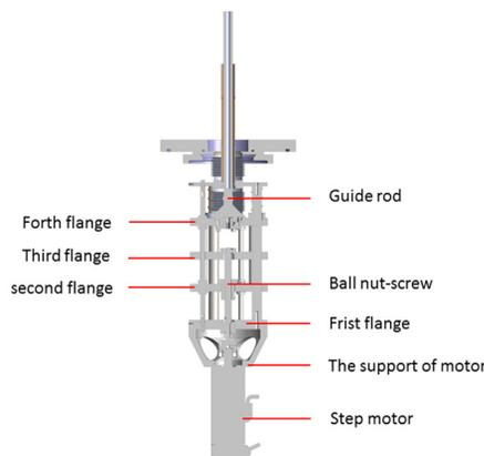
Figure 7: The sectional view of improved linear part.
