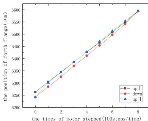
Figure 8: The curve of improved linear part.
