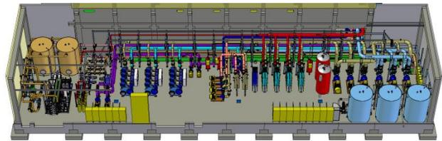
Figure 2: XHM pump house DESY Bahrenfeld, 3D model.
