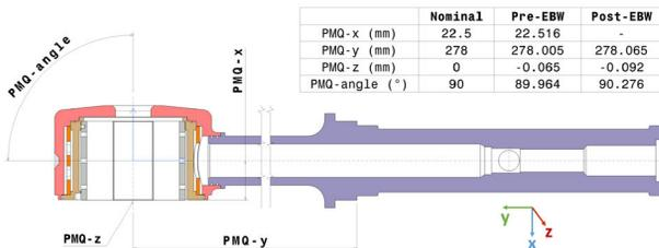
Figure 6: Measured PMQ axis position.
