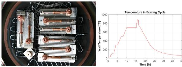
Figure 5: 8 DTs batch inside INFN-LNL brazing furnace (left) and his thermal cycle (right).
