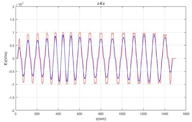
Figure 3: A comparison between the analytical fields used in BEAMPATH (blue) and the accurate 3D field generated by CST Microwave Studio (red).
