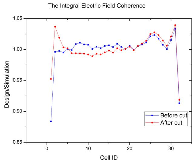
Figure 4: The integral field deviation between BEAMPATH and CST.
