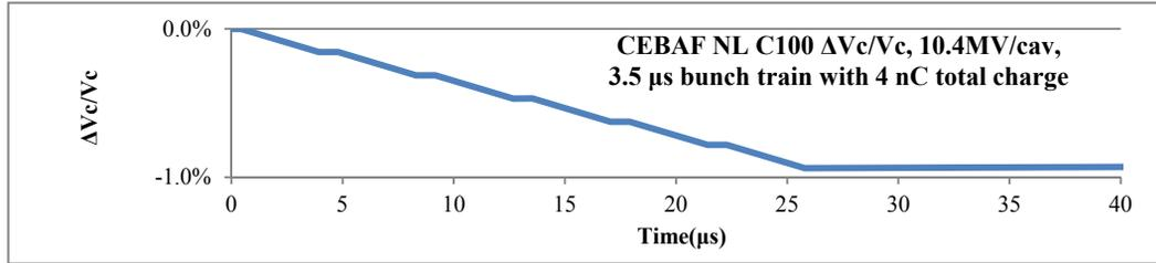
b) Detail of the transient beam loading when a bunch train passes through a C100 cavity 6 passes
