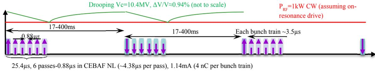
25.4μs, 6 passes-0.88μs in CEBAF NL (~4.38μs per pass), 1.14mA (4 nC per bunch train)
