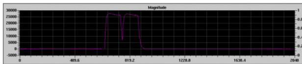
Figure 5. CEBAF NL M56 cavity signal for 100  $\mu\text{A}$  4  $\mu\text{s}$  bunch train accelerated through CEBAF for 1.5 passes.
