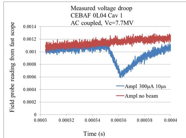
Figure 6. Measured voltage droop in CEBAF 0L04 Cav 1.
