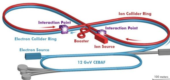
Figure 1: Conceptual layout of JLEIC.
