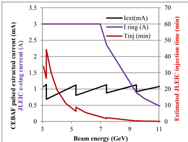
Figure 4. Beam current in the JLEIC e-ring and estimated injection time, no effective RF feed-forward/feedback.
