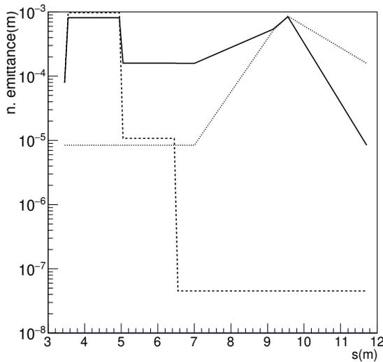
Figure 3: Emittance evolution of the simulation. The horizontal axis shows the distance from the cathode, and the vertical axis shows the normalized emittance in m.  $\epsilon_x$ ,  $\epsilon_y$ , and  $\epsilon_z$  are drawn with solid line, dashed line, and dotted line, respectively.
