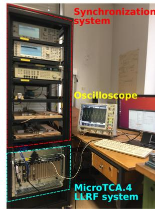
Figure 3: Front side view of the LLRF test setup.
