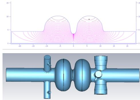
Figure 1: Two models of cERL injector cavity. Top is 2D cavity model and bottom is 3D cavity model.
