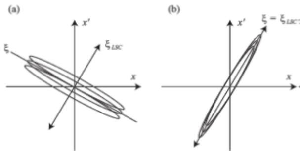
Figure 7: Diagram for compensating the emittance increased in the dispersion region by longitudinal space charge. (a) When the emittance deterioration amount becomes the maximum. (b) When the emittance deterioration amount becomes the minimum.
