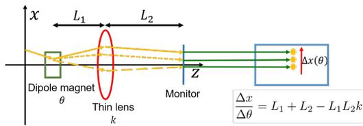
Figure 3: Schematic layout of single particle tracking.
