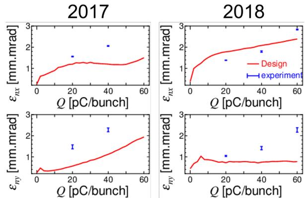
Figure 6: Emittance measurement result (left: 2017, right: 2018). The red line shows designed emittance value.
