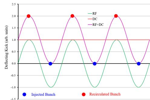
Figure 2: Kick in the rf separator with superimposed magnetic dipole, Fig. 2 from [3].
