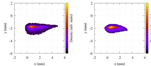
Figure 8: The undisturbed beamlet (left) and kicked beamlet (right), taken at the beam spot screen.
