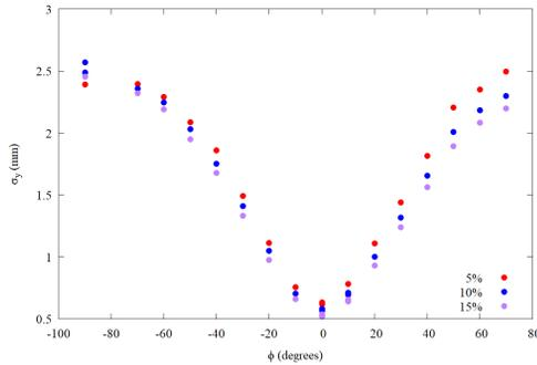
Figure 5: Measured *rms* vertical size,  $\sigma_y$ , on the longitudinal screen plotted as a function of degrees off-crest,  $\phi$ , for different thresholds.
