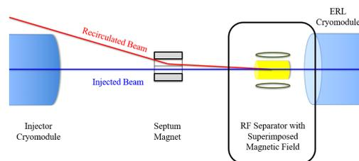
Figure 1: Layout of the “straight” merger concept, Fig. 1 from [3].
