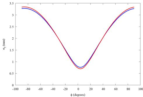
Figure 6: Simulated *rms* vertical size,  $\sigma_y$ , on the longitudinal (red) and beam spot (blue) screens plotted as a function of degrees off-crest.
