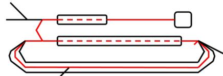
Figure 2: Scheme of the once recirculating ERL operation.
