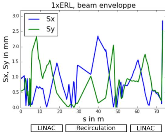
Figure 4: Simulation of horizontal ( $S_x$ ) and vertical ( $S_y$ ) beam envelopes for once recirculating ERL mode in x and y along the beam line.
