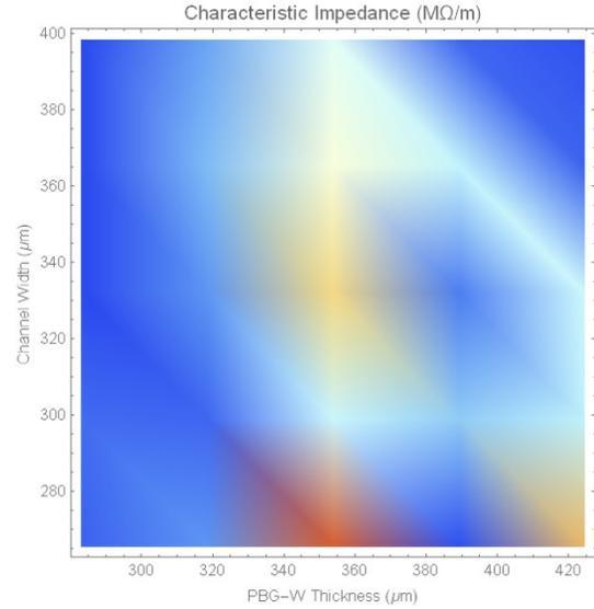
Figure 2: Variation of characteristic impedance with PBG-W thickness and channel width.
