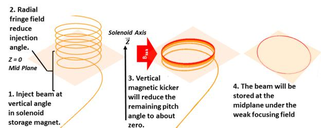
Figure 1: Layout of three-dimensional spiral injection scheme.
