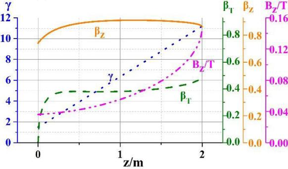
Figure 1: Dependence of initial guiding magnetic field  $B_z$ , electron energy  $\gamma$ , transverse velocity  $\beta_T$  and axial velocity  $\beta_z$  on axial distance  $z$  in CARA (from  $z=0$  to 2 m).
