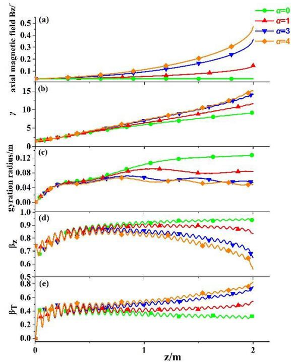
Figure 5: The (a) axial magnetic field  $B_z$  distribution along z axis under different  $\alpha$  value, dependence of (b) electron energy  $\gamma$ , (c) gyration radius  $\rho$ , (d) axial velocity  $\beta_z$  and (e) transverse velocity  $\beta_T$  on axial distance z under a tapered axial magnetic field shown in (a).
