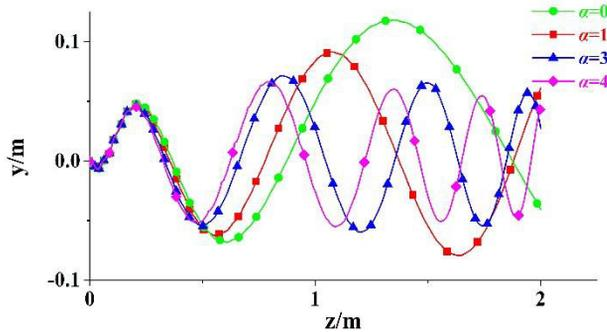
Figure 4: The projection of the motion of electron on the y-z plane under different magnetic field parameter  $\alpha$ .
