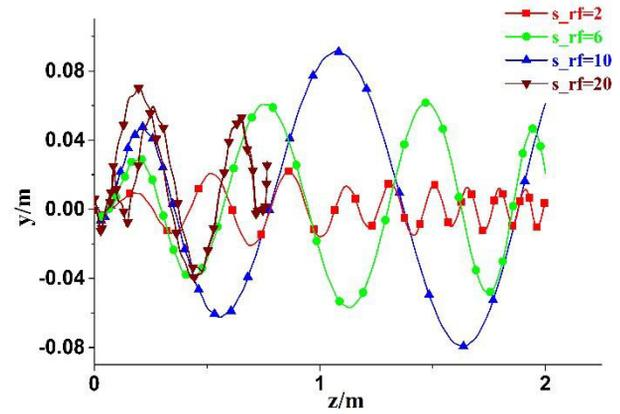
Figure 2: The projection of the motion of electron on the  $y$ - $z$  plane under different rf field strength  $S_{rf}$ .
