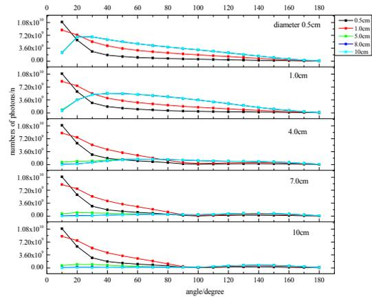
Figure 6: Photon angle spectrum produced in Ta targets with different diameters and thicknesses.
