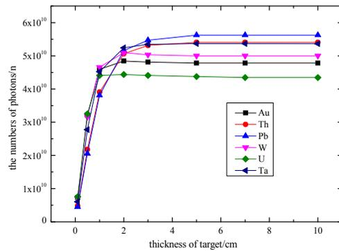
Figure 2: Calculation results of X-ray in heavy targets.
