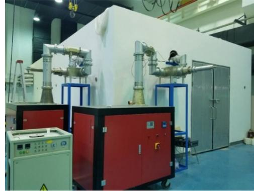
Figure 12: Tetrode-based RF system at site for XiPAF.
