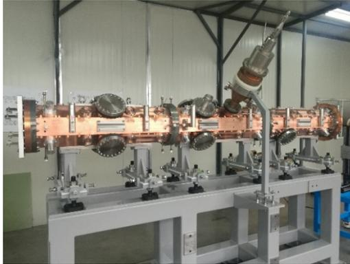
Figure 9: Assembled XiPAF RFQ for the tuning.
