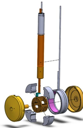
Figure 1: Drift tube structure.
