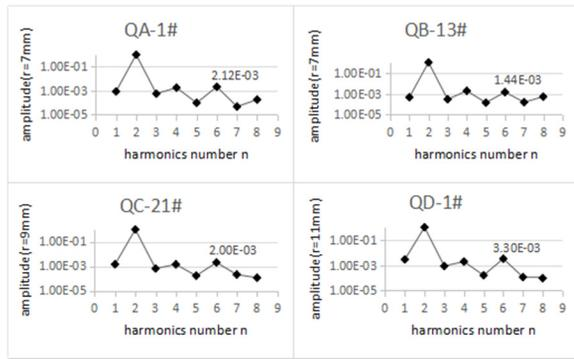
Figure 6: Higher-order harmonics of four types magnet.
