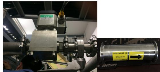
Figure 8: Flow meter and straight pipe.
