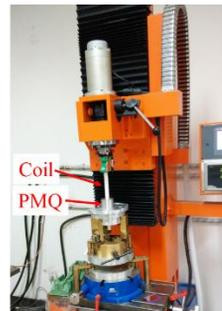
Figure 12: Rotating coil measurement.
