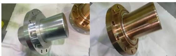
Figure 2: Two kinds of tuners (left: aluminium plunger tuner, right: copper tuner).
