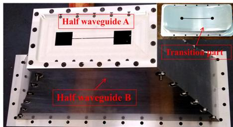
Figure 3: Split design of the cold model.
