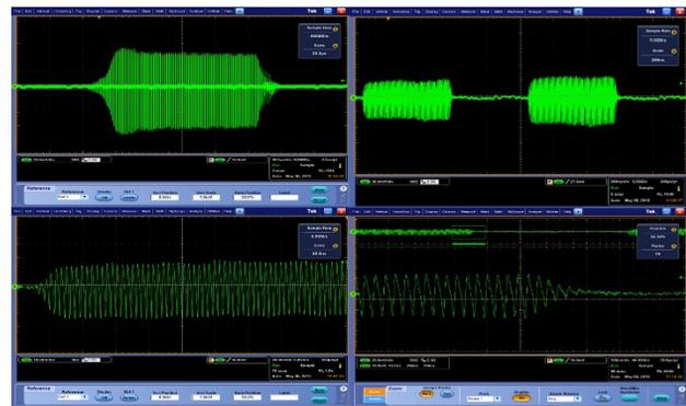
Figure 4: Beam signal of BPM after chopping. The upper plots: (left) the macro pulse of beam: 20µs/div; (right) the micro pulse of beam: 200 ns/div. The lower plots: (left) the rising edge of beam signal; (right) the falling edge of beam signal.
