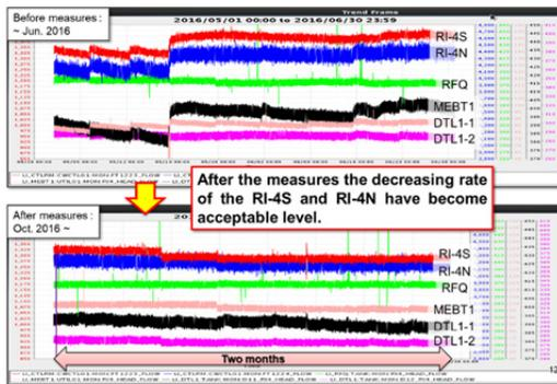
Figure 6: Cooling water flow rates for several cavity systems before (top) and after (bottom) the measure.
