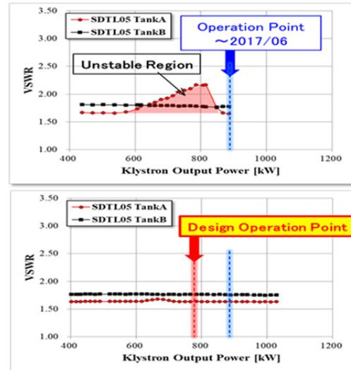
Figure 7: Voltage standing wave ratio for the SDTL#5 (Tank-A and B) cavities before (top) and after (bottom) the clean-up of the SDTL#05-tank-A cavity.
