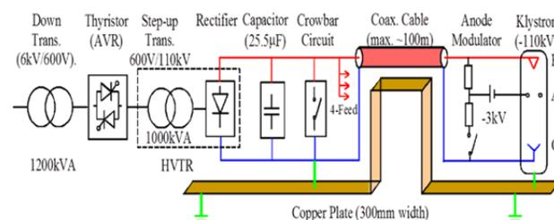
Figure 5: Circuit diagram of the HVDC.
