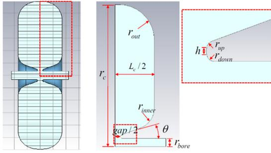
Figure 1: The parametric EM model of the nose-cone cavity.
