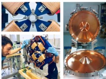
Figure 6: MEBT quadrupole with and without embedded BPM (top left, bottom left) and buncher (right).
