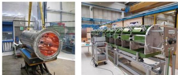
Figure 7: First copper plated DTL section at GSI (left) and aluminium mock-up model of the DTL (right).
