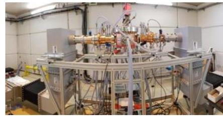
Figure 4: RFQ coupler conditioning test stand at CEA.
