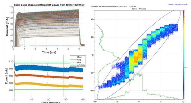
Figure 2: Ion source intra-pulse beam stability (top left), pulse-to-pulse stability (bottom left), and emittance at the RFQ entrance (right).
