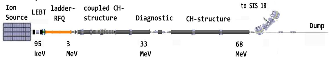
Figure 1: Layout of the FAIR Proton Linac.
