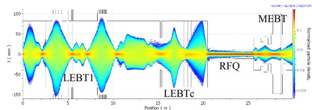
Figure 5: Density plot simulation of the  $^{18}\text{O}^{6+}$ .
