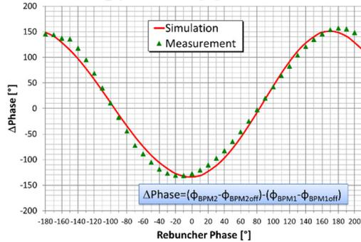
Figure 8: Discrepancy between the phase scan measurements (green dots) and the simulation (red line).
