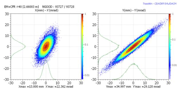
Figure 3: Calculated MEBT emittance –  $^{18}\text{O}^{6+}$ .
