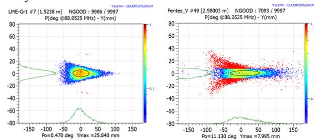
Figure 9: Left, phase – vertical position ( $\phi$ -Y plane) correlation created in the rebuncher. Right, same representation after the MEBT slits. Red particles are lost in the slits.
