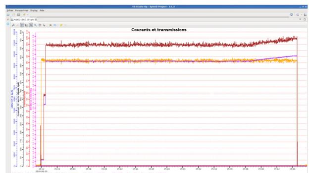
Figure 6: CW operation of the  $650\mu\text{A } ^{18}\text{O}^{6+}$  beam. At first at reduce 105 kV then at 113 kV. Red is the RFQ transmission, orange the beam current before RFQ, violet beam current after the RFQ.
