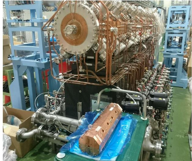
Figure 5: The 1300-MHz RFQ cold model together with a 324-MHz RFQ.
