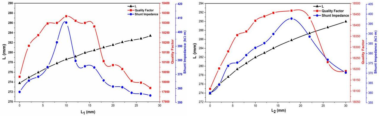
Figure 5: The variation of the lateral dimension (L), quality factor and shunt impedance of the bent-vane RFQ as the functions of the parameters of the cross-section profile (Only presenting two parameters).
