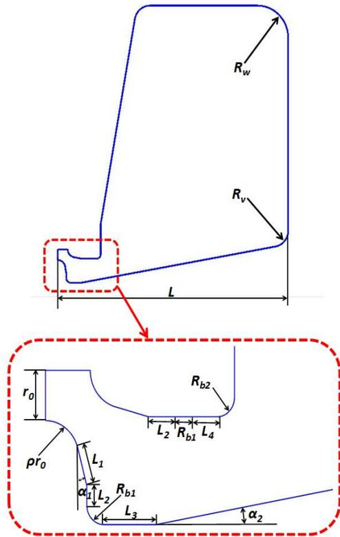
Figure 2: The cross-section profile of the bent-vane RFQ.
