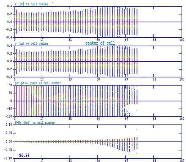
Figure 1: Beam dynamics simulation of the bent-vane RFQ (RFQGen).
