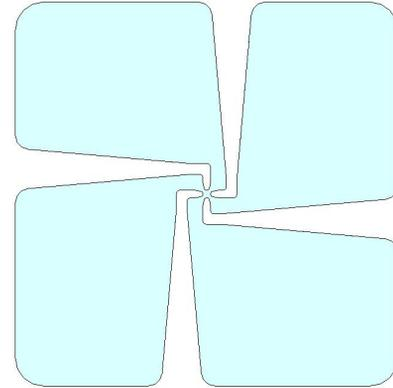
Figure 4: The slice model of the bent-vane RFQ.
