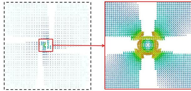
Figure 3: The electric field distribution of the bent-vane RFQ.
