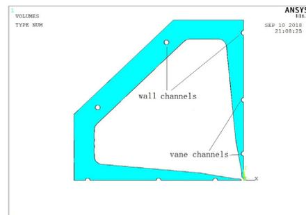
Figure 2: Thin slice model with water cooling channels.
