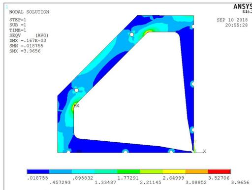
Figure 4: The von-Mises stress distribution of the RFQ.
