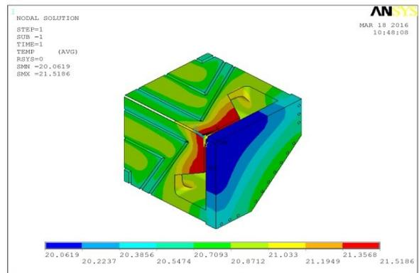
Figure 6: The temperature distributions of the RFQ undercuts.
