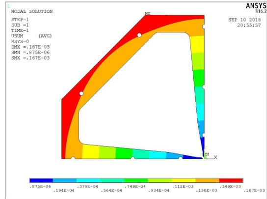
Figure 5: The displacement distribution of the RFQ.
