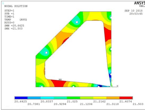
Figure 3: The temperature distribution of the RFQ.
