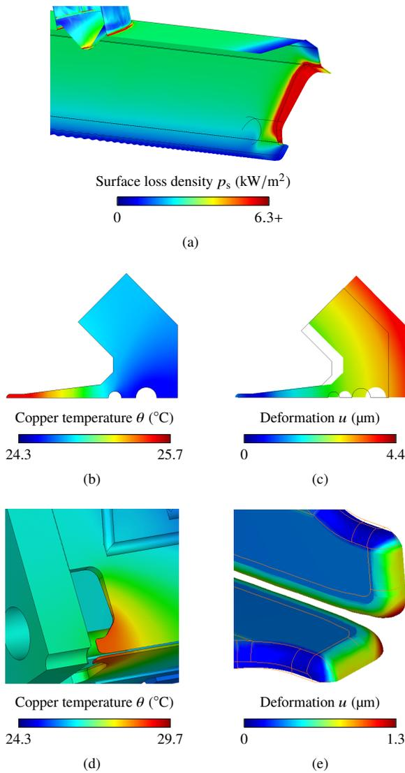
Figure 5: Thermal simulation results for nominal parameters (2.5% duty cycle,  $\theta_w = 22^\circ\text{C}$ ,  $v_w = 1\text{ m/s}$ ). (a) Power loss  $p_s$  on cavity surface. (b) temperature  $\theta$  and (c) deformation  $u$  of the octant-symmetric cross section; (d), (e) respective results around the vane nose.
