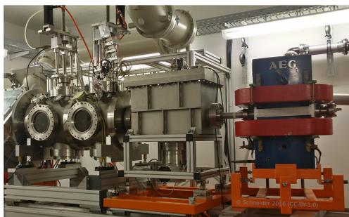
Figure 1: The diagnostic train in operation (left to right): emittance meter – beam dump – momentum spectrometer.
