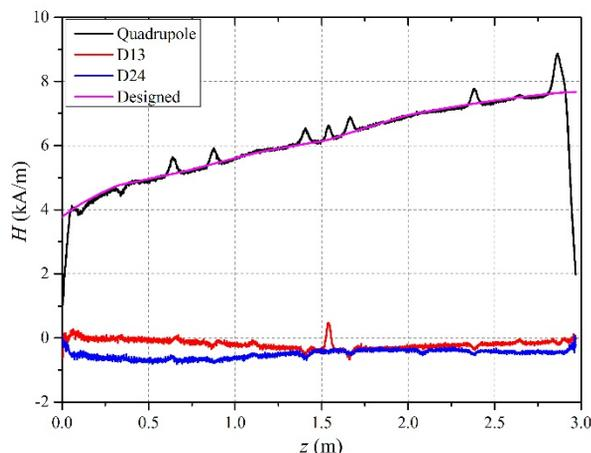
Figure 3: Normalized field distribution of the quadrupole and dipole modes after pre-braze tuning (22 °C, and 42% humidity).
