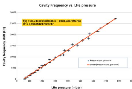
Figure 5: Cavity frequency shift as a function of helium pressure from 50 to 800 mbar.
