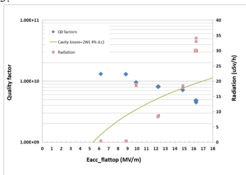
Figure 3: HB cavity package performance as a function of accelerating gradient.
