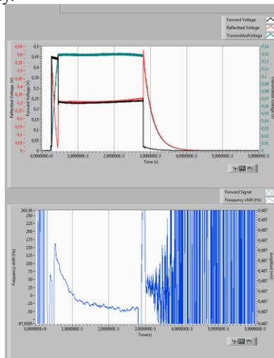
Figure 4: Top: Forward (black), reflected (red) and transmitted (green) signal during 2.55 ms pulses. Bottom: Dynamic Lorentz detuning of ESS HB elliptical cavity at 15 MV/m.
