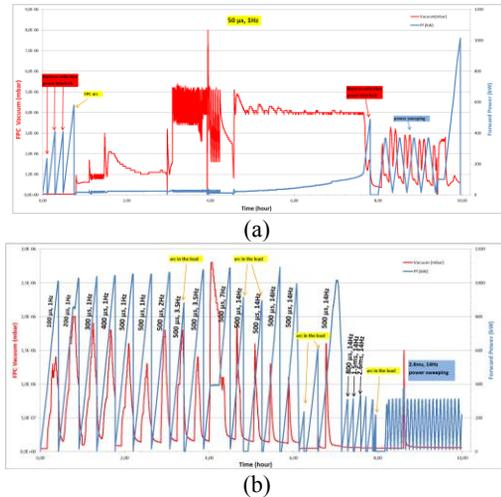
Figure 2: (a) HB cavity RF conditioning history with 50  $\mu$ s and 1 Hz repetition rate; (b) HB cavity RF conditioning history with longer pulse duration at different repetition rate, where the blue curve represents the RF power and the red one represents the coupler vacuum.
