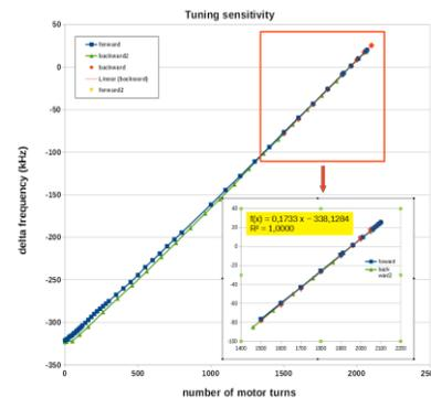
Figure 6: Tuning sensitivity of ESS HB elliptical cavity.
